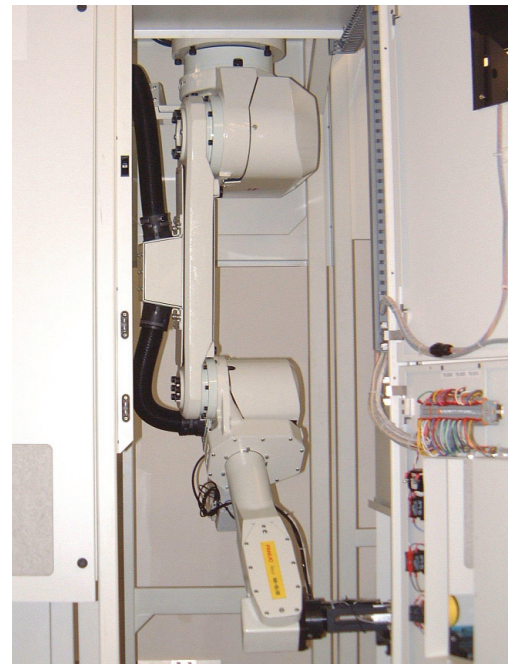
M-6iB within FOUF buffer invert-mounted for increased cell layout flexibility
