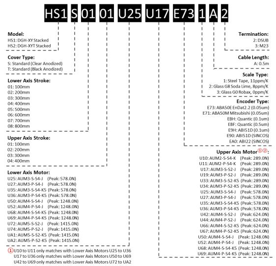
②For DGH-XYT Stacked, Theta Motor used is tagged to the Upper Axis Motors chosen: U10 to U36: AXD160-55 (Peak: 19.07Nm) U42 to U69: AXD200-65 (Peak: 42.78Nm)
