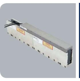
Parker Trilogy's I-Force ironless linear motors offer high forces and rapid accelerations in a compact package. With forces ranging from 5.5 lbf (24.5 N) - 197.5 lbf (878.6 N) continuous up to 5.5 lbf (24.5 N) - (883 lbf (3928 N) peak, the I-Force family offers a superior combination of performance and size.
