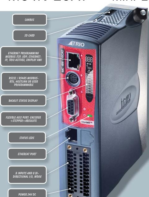
The MC4N-ECAT is a high performance Motion Coordinator that is dedicated to running remote servo and stepper drives via the EtherCAT real time automation bus. It is based on an up-rated version of the 532MHz ARM 11 processor which makes it ideal for high axis count machines or robotic applications.
