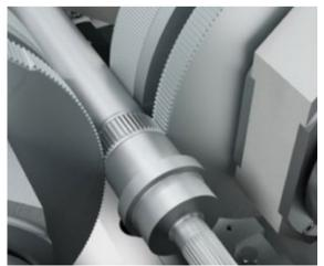
Galaxie  $^{\rm @}$  in a spline rolling machine – faster processing speeds increase productivity by 40 %
