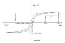
If the input shaft is locked, the gearbox is continuously loaded and relieved at the output in both directions up to a defined torque. The torsional angle is plotted against the torque. This yields a closed curve from which the → torsional backlash and → torsional rigidity can be calculated.
