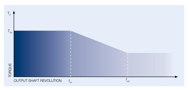
Torque in line with the relevant output shaft revolution
